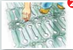
Clip plates together, cut plates with jigsaw if necessary
